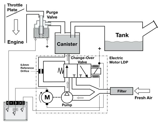
Once the test is concluded, the ECM stops the pump motor and immediately de-energizes the change over valve. This allows the stored pressure to vent thorough the charcoal canister trapping hydrocarbon vapor and venting air to atmosphere through the filter.
