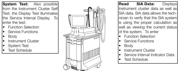
**Test Modules:** Problems with the SIA System can be diagnosed using fault or Symptom driven test modules. To begin diagnosis: • Short Test
