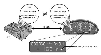
The data is compared each time KL 15 is switched on. If the data does not match, the manipulation dot in the mileage display block will be illuminated.
