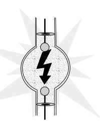
*Starting Phase:* The bulb requires an initial high voltage starting pulse of 18-25kV to establish the arc.
