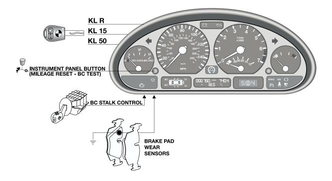
**INSTRUMENT PANEL BUTTON -** The reset button is used to reset the trip - odometer as in the past. It will also display the mileage, if pressed with the key switched OFF. This button is also used for the Base BC/instrument cluster test functions outlined on page 15.
