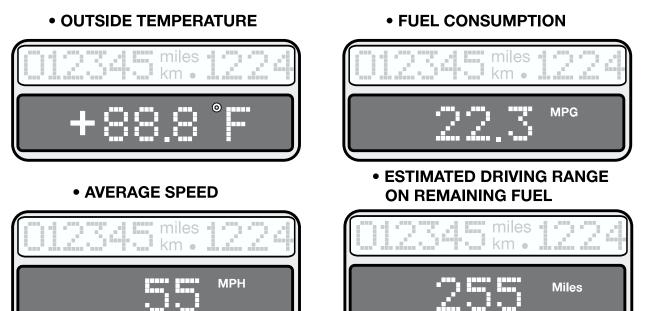
The current time is always displayed when KL R is switched on. Any other BC display value can be called up by pressing the turn signal lever.
