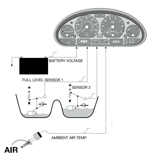
**OUTSIDE TEMPERATURE SENSOR** - A NTC sensor is used to measure the ambient temperature. The signal is processed by the cluster and passed out over the K Bus to modules requiring this input for processing.
