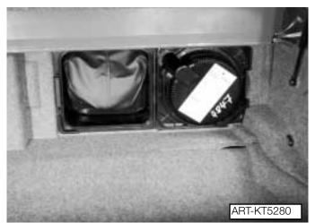
The subwoofer is hinged so that it will swing to the side when the ski bag is used. A magnet on the subwoofer cover will hold the subwoofer in place against the rear bulkhead while the ski bag is being used.
