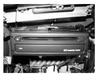
There are two different hardware versions available dependent on the angle of installation in the vehicle (horizontal or vertical). The Mk-3 is compatible with both board monitor or MIR display units. (See workshop hints for configuration instructions)
