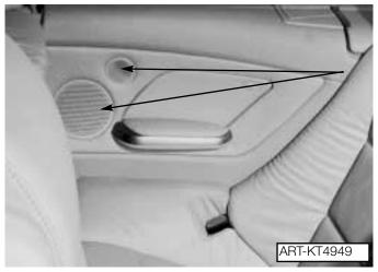
Speaker and component locations will vary depending on the type of sound system installed. Four rear speakers are mounted in the rear side trim panels, two on each side (one wide band 130 mm and one tweeter dome).
