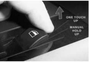
Momentarily pushing the switch to the second detent and releasing provides an additional ground signal on the second wire requesting the "one touch mode", operating the window motor automatically. The motor runs the window down until it reaches it's end stop.
