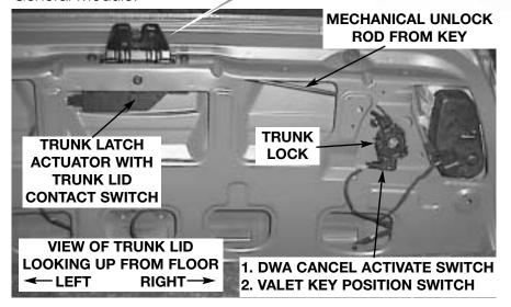
Valet position switch: With the key lock in the valet position, this switch provides a ground signal to the GM.
