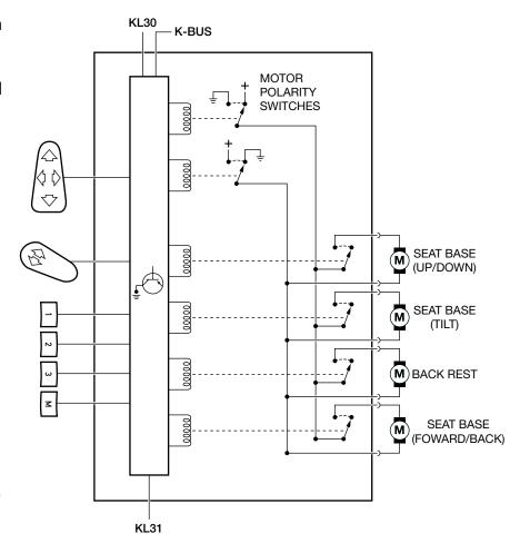
The multiplexer control activates the polarity contacts and then the individual motor contacts to run the motors individually.
