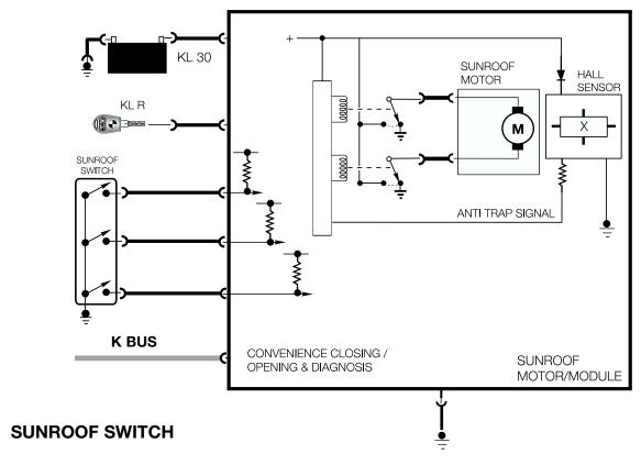
Mounted in the sunroof motor trim cover is the sunroof switch. Also similar to previous systems, the switch provides coded ground signals for system operation.
