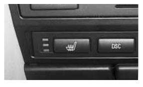
stage 3. The top and middle LEDs are off and the heating elements are regulated to an output temperature of 95°F.
