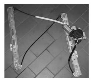
The windows are run to their limit stops which is detected by an amperage increase in the control circuit. Additionally, the window run cycle is limited to an 8 second duration if in case the amperage increase is not detected or there is a malfunction with the regulator.
