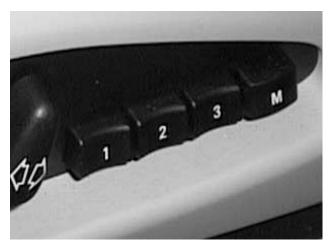
The stored position can be recalled at any time by pressing the appropriate memory location button (1-2-3).
