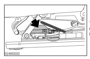
The memory control module for the seat is mounted under the seat base on the seat frame.
