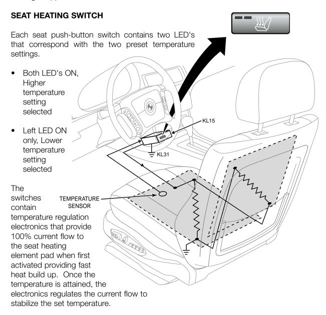
The switches provide operating current to the seat heaters until switched off. There is no preset time limit of operation.
