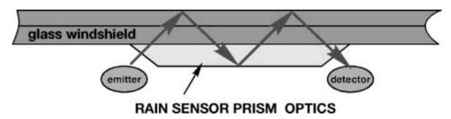
The density of water is closer to that of glass than air. When rain starts to accumulate in the sensor monitoring area, it causes part of the infra red beam to extend past the outside surface of the glass and into the rain drop. When this occurs, the beam is refracted and only part of the beam returns to the detector diode.
