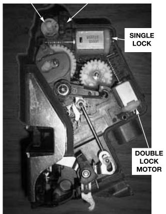
**ACTUATOR IN UNLOCKED POSITION**
