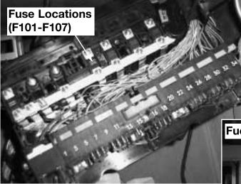
The electronics carrier is located forward of the glove box. It contains the following components as noted in the photograph. Located above the fuse panel are additional high amperage power distribution fuses (F101-F107).
