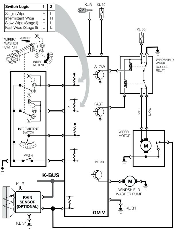
**WINDSHIELD WASHING:** Pulling the Windshield Wiper Switch rearward closes the "windshield wash" contacts and provides a switched ground input to the GM. The GM activates the windshield washer pump directly via a power output final stage transistor.
