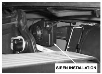
The rechargeable battery will allow the siren to sound if it or the vehicle's battery is dis-connected. The siren battery is recharged, from the vehicle's battery when DWA is not in the armed state.
