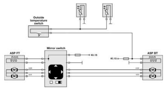
the heating element in the driver's door mirror. Passenger door mirror heating element power supply is provided directly. The mirrors are heated regardless of outside ambient temperature. The heating element resistance produces a mirror temperature of approximately 60°C.
