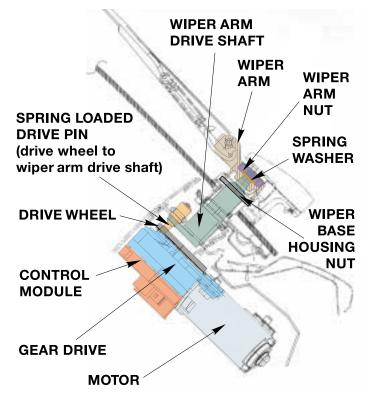
The wiper pivot bearing, wiper shaft and wiper arm are mounted on the rear window. A mechanical coupling is used to connect the two components as on the E39 wagon.
