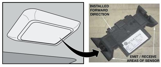
The interior sensor is mounted in the center of the headliner panel even with the "B" pillar. Due to the design of the vehicles interior, the sensor is uni-directional and must be installed in the proper direction to ensure proper operation of the system (trim cover ensures directional installation).
