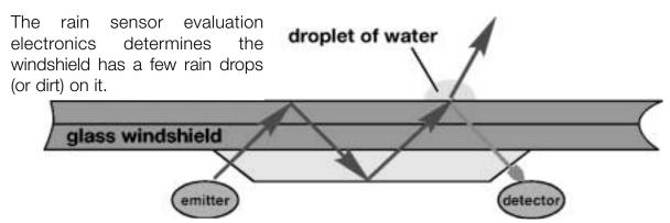
The intensity of the returned infra red beam diminishes proportionally with an increase of water droplets. The rain sensor control module generates a signal proportionate to the amount of rain on the windshield and broadcasts it to the GM V via the K bus.
