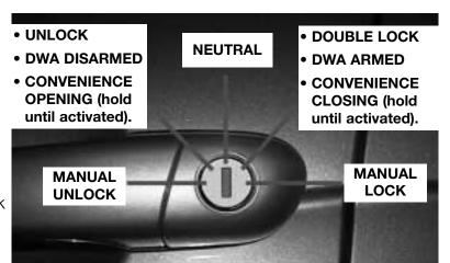
The GM monitors these key positions over two wires. The signals are generated by two hall effect sensors (Hall Sensor 1 & 2) located in the actuator.
