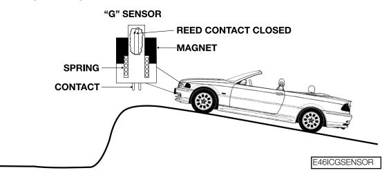
However, if the vehicle becomes airborne and weightlessness occurs, the spring will force the magnet up and the reed contact will open. This will signal the electronics of the sensor to trigger the solenoids and the roll bar will deploy.
