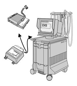
Typical with any airbag, it is to be replaced as a unit after deployment. This is the same for ITS assemblies and the BST.
