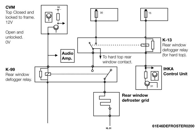
Relay K-13 also supplies KL 30 to relay K-99 when the button is pressed on the IHKA control panel. Relay K-99 is energized when KL R is switched ON and the soft top is closed and locked to the windshield frame. This allows the grid in the soft top window to be heated. When the soft top is lowered, KL R to relay K-99 is interrupted by the CVM to prevent the grid from heating when the top is lowered into the storage compartment.
