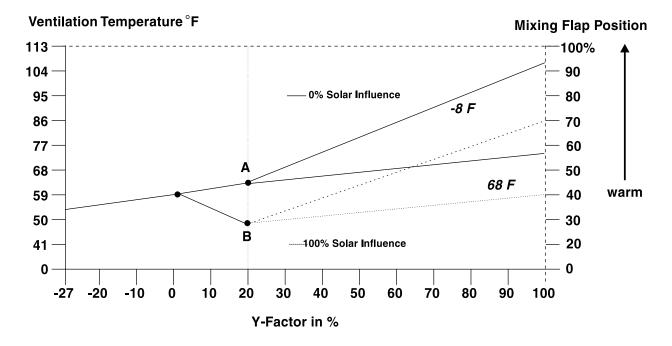
To illustrate the influence of the solar sensor on the mixing flap position, the Y factor remains constant at 20%.
