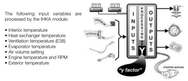
The processed variable "Y-factor" is determined by using the above inputs. The Y-factor then represents how much adjustment is necessary by the IHKA module to achieve the set temperature.
