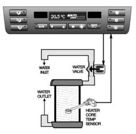
SERVICE STATION FEATURE - The "Service Station" feature introduced with the E38 IHKA is integrated into the E46 IHKA. This prevents the heater core from being flooded with hot coolant when refueling the vehicle.
