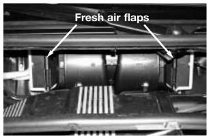
When the key is turned off with re-circulation on, the fresh air flaps will open. Re-circulation memory in the IHKR control unit is 15 minutes. If the vehicle is started within 15 minutes the re-circulation setting will be restored.
