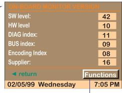
Key Functions tests the key input on the BMBT. Input status (1-25) will display in the window.
