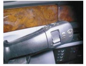
Pressing the wiper stalk forward to the first detent activates the rear wiper in the intermittent mode. The timed interval is approx. 7 seconds. The full sweep and park positions are recognized by the two hall sensors on the motor gear assembly. If the wiper is switched OFF, the wiper blade will return to the park position.
