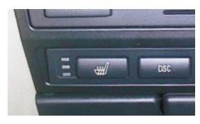
Pressing the button a second time provides stage 2. The top LED switches off and the heating elements are regulated to an output temperature of 102°F. Pressing the button a third time provides stage 3. The top and middle LEDs are off and the heating elements are regulated to an output temperature of 95°F.
