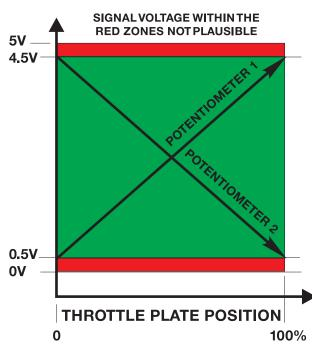
Pot signal 1 is the primary signal, signal 2 is used as a plausibility cross-check through the total range of throttle plate movement.
