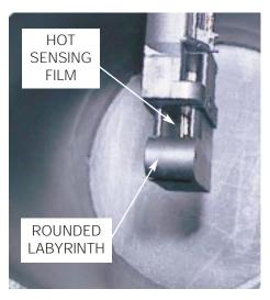
An additional improvement of the HFM 5 is that the hot film element is not openly suspended in the center bore of the sensor as with previous HFMs. It is shrouded by a round fronted plastic labyrinth which isolates it from intake air charge pulsations.
