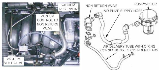
The DME ME7.2 control unit controls the vacuum vent valve and the secondary air injection pump relay separately but simultaneously.
