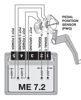
The PWG provides two separate variable voltage signals to the ME 7.2 control module for determining the request for operating the Electric Throttle Valve (EDK) as well as providing a kickdown request with automatic transmission vehicles.
