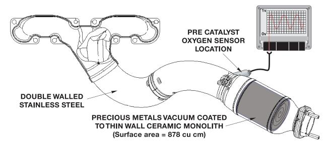
The Bosch LSH 25 oxygen sensors are carried over from the M62 engine and provide the familiar "swinging" voltage signal (0.2 - max lean to 0.8 - max rich) representing oxygen content in the exhaust gas.
