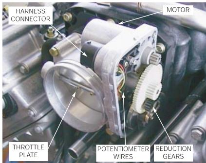
Engine idle speed control is a function of the EDK. Therefore, the M62 TU does not require a separate idle control valve. This ME 7.2 controlled sub-system is described in the Electric Throttle System Functional Description (page 32) and in the ME 7.2 Input/Output signal sections further on.
