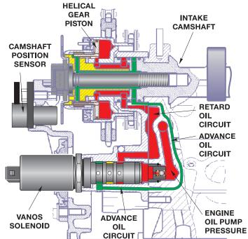
**OIL DISTRIBUTION FLANGES:** The oil distribution flanges are bolted to the front surface of each cylinder head. They provide a mounting location for the VANOS solenoids as well as the advance-retard oil ports from the solenoids to the intake camshafts.
