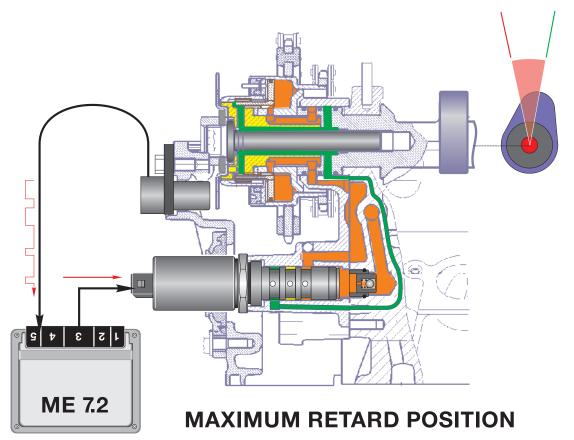
• **Top of next page**: As the Pulse Width Modulation (PWM) increases on the control signal, the valve progressively opens the advance oil port and proportionately closes the retarded oil port.
