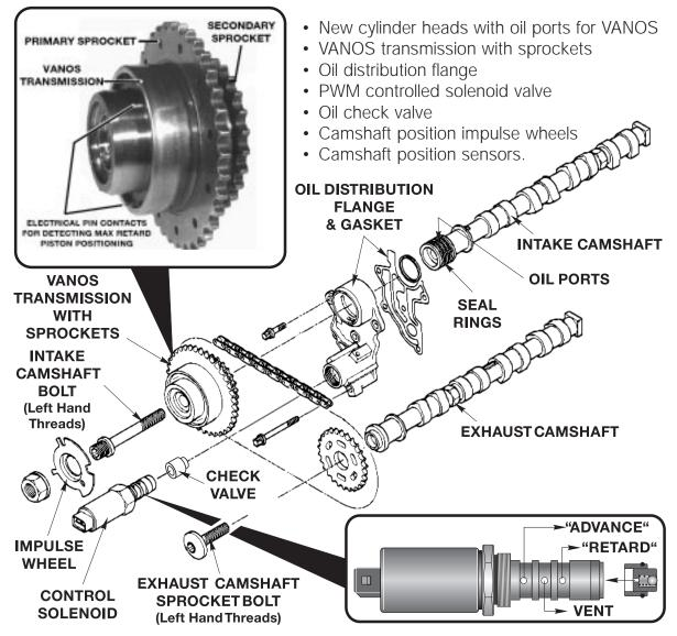
**VANOS CONTROL SOLENOID & CHECK VALVE:** The VANOS solenoid is a two wire, pulse width modulated, oil pressure control valve. The valve has four ports;
