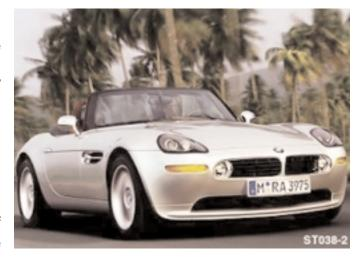
The complete body of the Z8 is made of aluminum. The body is produced in the Dingolfing plant and the vehicle is then finished built as a limited production in Munich plant.
