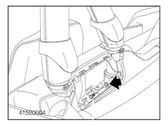
The roll bar has been removed from the mounting sleeves to allow visibility of the single mounting bolt on the right, and the four bolt locating plate on the left.
