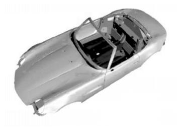
In addition to the bolt on panels shown in this illustration, compound outer panels such as door, hood, and trunk skins are bonded to their support frames.
