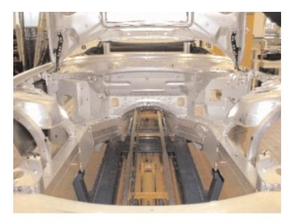
The aluminum strut tower structure can be seen here on the right which is supported by two channel braces that connect with the upper support rail.
