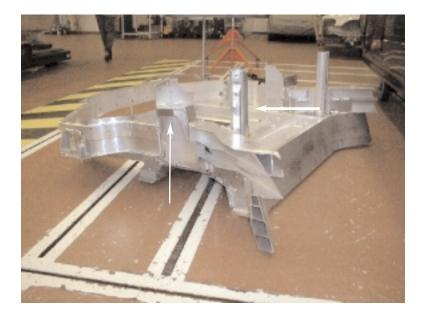
The left rear frame structure shown on the right highlights the upswept rear frame rail and the mounting point for the rear impact absorber.
