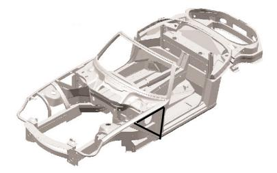
The front structure illustration on the right highlights the additional frame support behind the front bumper assembly.
