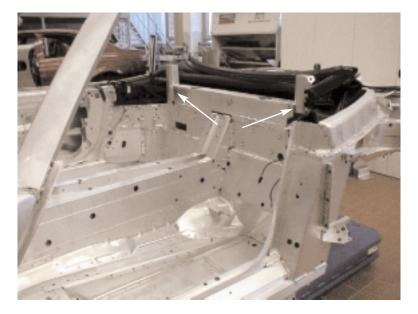
The rear frame section (right side shown) points out the rear strut tower support and the integral roll bar mounting.
