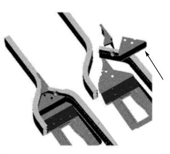
The frame and floor pan assembly illustration on the right shows additional triangulation reinforcement pieces.
