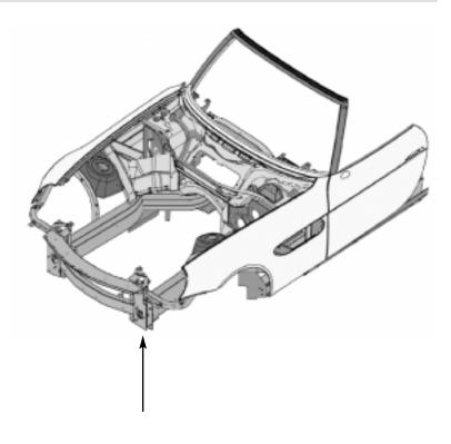
The engine compartment structure shown in this actual view reveals the massive frame rail size.
