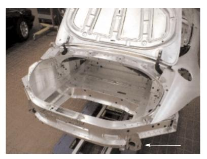
The luggage compartment floor insert is a bolt in plastic tray that holds the battery, tool kit, and antenna amplifier.
