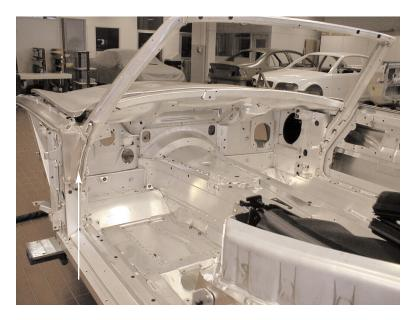
The aluminum "space frame" with joint connection is highlighted on the right.
