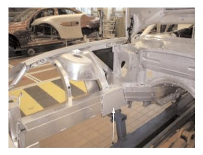
The left rear floor section shown here reveals the inner frame rail mounting to the rear support beam.
