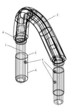
The rollbar is connected to the body mount by a sleeve.
