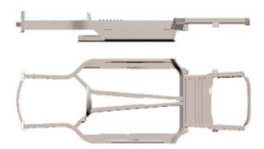
Using the "Y" structure provides the additional strength needed to compensate for the lack of a roof (open roadster).
