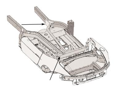
Shown on the right is the windshield frame structural mounting and engine compartment bulkhead assembly.
