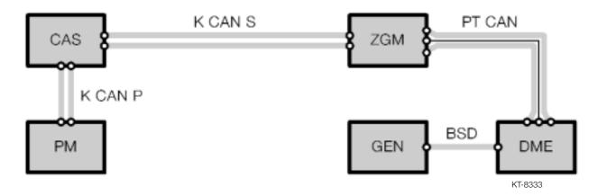
The Power Module detects the temperature of the battery and places the instruction "Increase charge voltage" on the K-CAN Periphery. The Car Access System (CAS) passes the message on to the K-CAN System bus.
