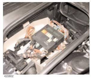
Right side engine compartment inside the Integrated Voltage supply Module (IVM)
