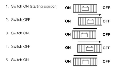
The function is cancelled by: "terminal 15 On", switching the battery switch from "OFF" to "ON" or failure of the battery voltage to reach 12.6 V after 6 hours of charging.
