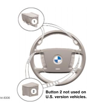
"Low" program: Operating the two buttons on the face of the steering wheel signals the EGS (TCM) to perform a down-shift.
