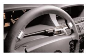
In addition to the MFL buttons familiar from the E38, the transmission can now also be shifted from the steering wheel. The left-hand group of function buttons on the steering wheel are used to control the functions: voice input, audio/nav/telephone(volume), telephone (send/end call).
