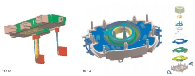
Integrated Steering Wheel Electronics Module located in steering wheel.
