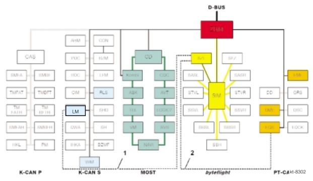
The SZL is a satellite of the overall ISIS system (Intelligent Safety and Integration System) on the *byteflight* bus system.
