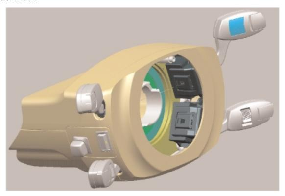
The electrical steering column adjustment incorporates the comfort entry function. The steering wheel can be adjusted fore and aft and vertically to suit the driving position.
