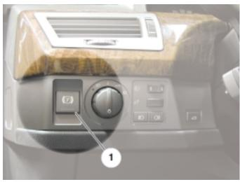
When the vehicle is stationary with the ignition switched on, the parking brake is applied or released by pressing the button.
