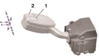
The top switch (2) activates the board computer display on the instrument cluster below the tachometer. This shows information such as average fuel consumption and average speed. The lower switch (1) activates the On-Board Computer display on the instrument cluster below the speedometer. This shows information such as fuel level and range.
