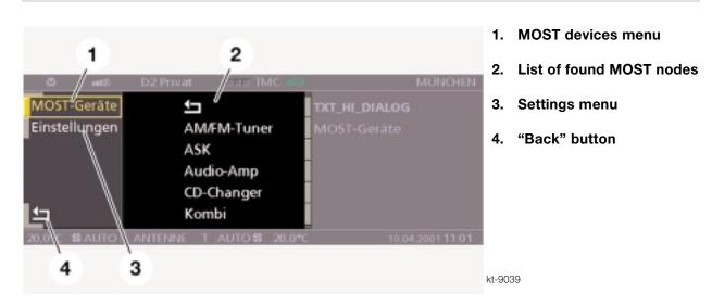
The Control Display knows how many MOST nodes there are, i.e. how many MOST nodes there are on the MOST ring bus. When retrieving the list of MOST control units fitted, the Control Display waits for a response from each MOST node. Every control unit on the MOST bus contains a MOST communication chip.
