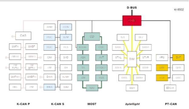
The Control Display communicates via the MOST bus system with all other components on the MOST bus.
