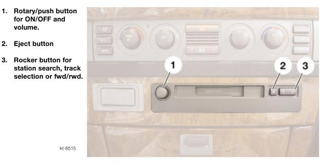
The control panel and the ASK control module are a single unit. The control panel incorporates the main rotary/push-button control for switching on all audio sources. It is also the volume control.
