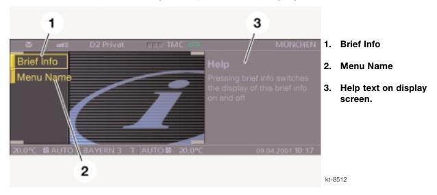
The help is activated by selecting the "Brief Info" button with the Controller and then depressing the Controller to confirm the selection.
