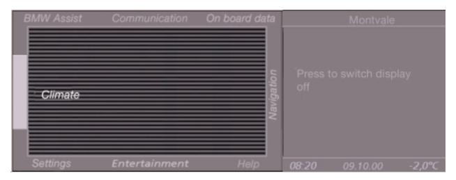
The button for the selected menu is visually highlighted and the menu name displayed in the control area. This applies only if the function Menu Name has been activated in the Help system or if the Controller is held in the deflected position for more than 1 second.
