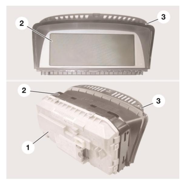
A 16-bit processor is responsible for communication (gateway function) between the MOST and K-CAN SYSTEM bus systems, it also performs the tasks of diagnosis processing and illumination dimming.
