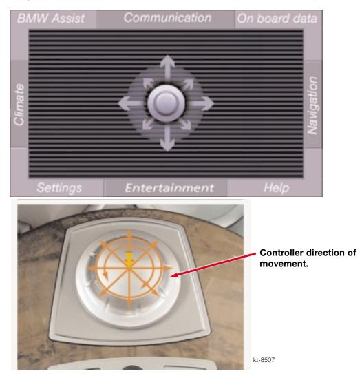
The 8 main directions of movement of the Controller are scanned by a switch unit. That switch unit consists of 8 individual switches. They are positioned at 45 degrees to each other.
