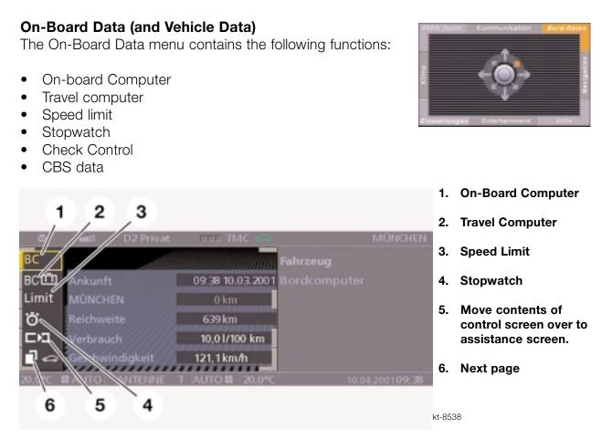
The button with the arrow symbol can be used transfer the current display in the control area to the assistance screen.
