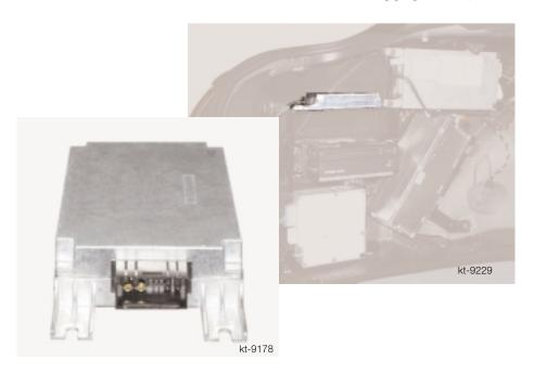
The SVS control unit has one 12 pin ELO connector that supplies KL 30, KL 31 and the two MOST connections.
