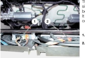
The satellites of the driver and passenger side are identical. The satellite is located below the seat frame between the seat rails. It is fitted with the seat module beneath a cover in a plastic tray.
