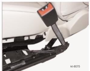
There is also earlier restraint and thus earlier binding to the vehicle. The seatbelt tensioner forms a unit with the seatbelt buckle. It consists of an ignition stage, generator, plunger and cable. The belt buckle switch is integrated in the seatbelt buckle.
