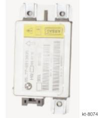
The SBSL satellite is connected to the SIM via the *byteflight*. The power supply of the satellite is also from the SIM and it is buffered by the memory backup capacitor.
