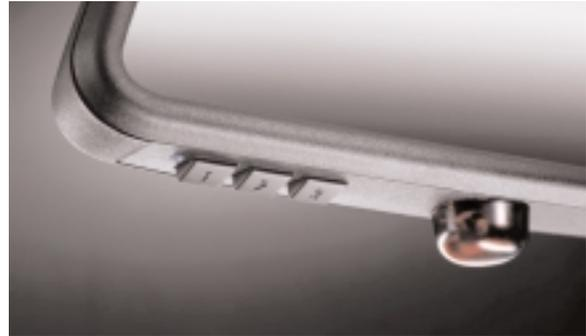
The signal of an original hand held transmitter can be programmed to one of the three channel buttons. The device is operated with the programmed channel button. The integrated universal remote control uses radio frequencies only (not infrared). Transmission of the signal is indicated by the indicator LED.
