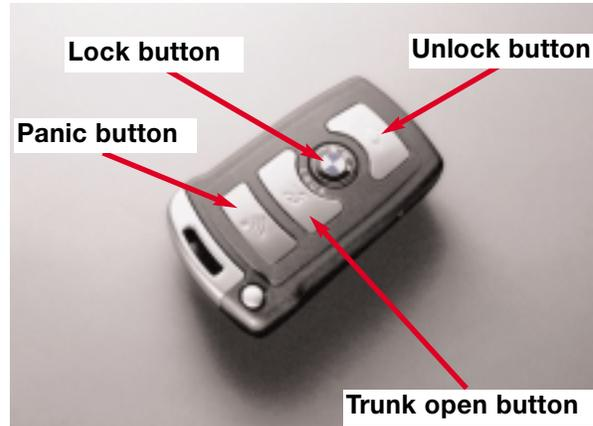
The rechargeable battery voltage is monitored independently by the Remote Control and signaled to the CAS.
