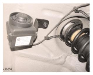
Detected alarm triggers are communicated to the DWA control unit, which then activates the alarm.
