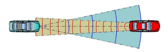
The relative speed difference between the vehicle and the object is determined by the Doppler effect of the Radar. The Doppler effect was named after Christian Doppler, who first came up with the idea in 1842. He thought that the frequency of sound (or in the case of radar, radar waves) waves would change if either the source or the observer was moving. If they were approaching, the frequency would be higher; if they were moving away, the frequency could be lower.
