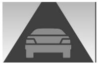
**Take Over Request** Vehicle in display is in triangle and Flashes: Driver should intervene by braking or taking evasive action as required. ACC cannot set following distance.
