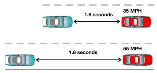
Constant interval based on seconds, distance changes based on speed.
