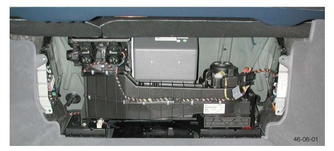
The control and integration of the rear compartment air conditioning system in the IHKA refrigerant circuit is designed so that independent operation is possible for either the front or rear unit.
