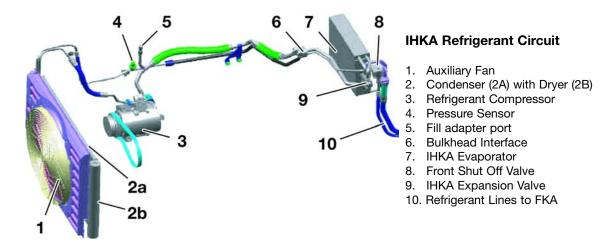
The rear compartment air conditioning system (FKA) is connected to the refrigerant circuit of the IHKA. The two circuits are isolated by means of two shut-off valves that are fitted only in connection with the rear compartment air conditioning system. The shut-off valves are fitted in the pressure line ahead of the respective expansion valves of IHKA and FKA.
