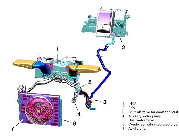
The rear compartment air conditioning system is operated by means of:
