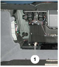
The Condensation Water Drain below the evaporator is designed to ensure the condensation water is drained off reliably even with the vehicle in extreme positions.
