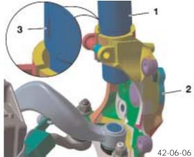
Spring Strut, Hub Carrier, and Wheel Bearing
