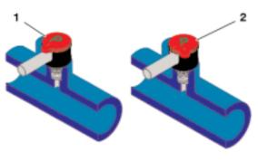
Prior to reconnection, the cap must be reset to the locked operating position (1) and should be plugged into the connection only in this position.
