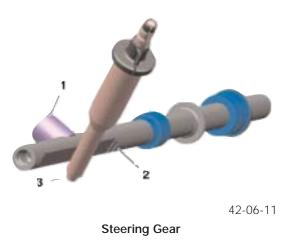
With larger dimensioning, the rack and pinion steering system is used in the E65. The thrust piece required for automatic play compensation is lengthened and equipped with a stronger spring. The thrust piece contains integral lubrication pockets where it contacts the rack for longevity and noise reduction.
