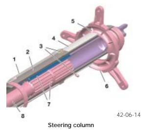
The compression movement begins when the three plastic pins shear under an axial force of approximately 3 kN.
