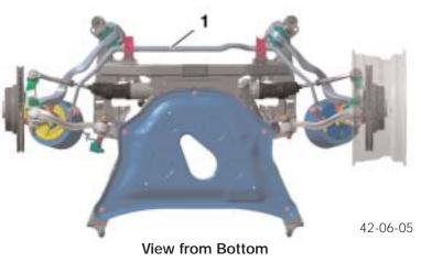
Spring Strut, Hub Carrier and Wheel Bearing: The twin tube gas pressurized shock absorbers and the hub carrier are bolted together. The tube is made of aluminum and has a locating tab on the side which is used to align it into the hub carrier in the correct position.
