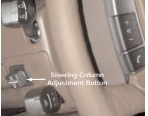
The steering column is automatically moved to the uppermost forward position to provide easy entry and exit from the driver's seat.
