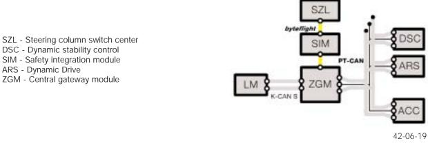
Steering Angle Sensor Communication Link
