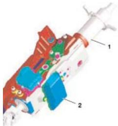
The CIM is linked to the K-CAN S Bus for communication with other control modules. The ZGM provides the gateway for diagnostic communication.
