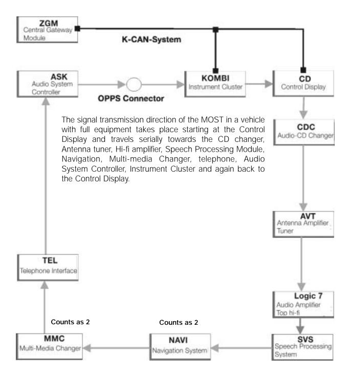
Important!!! The component sequence of the MOST controllers in the ETM is incorrect when it comes to signal transmission direction. The correct sequence is indicated above!
