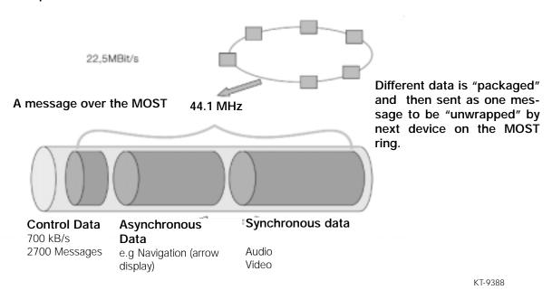
The control data controls the functions and devices in the network. The information can be compared to CAN bus data.
