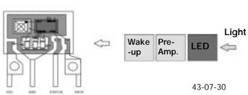
An interface that converts the optical signal into an electrical signal
