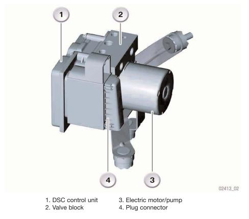
In a DSC control operation, the braking pressure is built up with the aid of an electric motor. A pressure sensor integrated in the valve block senses the braking pressure established when the driver applies the brake.
