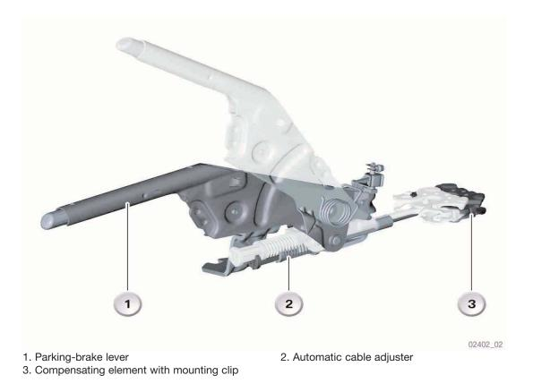
The mounting clip locks the cables in the compensating element. The duo-servo brakes correspond to the duo-servo brakes of the E65 (dia. 185 x 30 mm).
