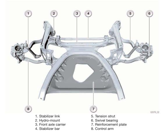
Axle alignment is performed at the tie rods. If necessary, the camber is corrected by removing the pin on the upper support bearing.
