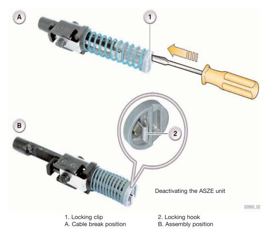
The cables can now be disconnected from the duo-servo brakes. To be able to disconnect the cables, it is necessary to remove the mounting clip.
