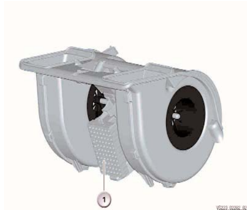
1. Blower controller on blower motor
