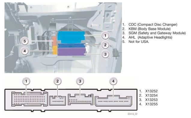
(X13252 54-pin, X13254 3-pin, X13253 13-pin, X13255 6-pin) and an operating voltage range of 9-16 Volts. The KBM is internally protected against shorts to terminal 30 or 31 and equipped with reverse polarity protection.
