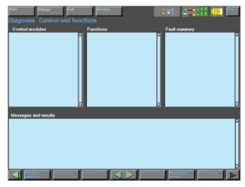
If a short test was not performed from the vehicle identification screen, no modules will appear under the control modules column.
