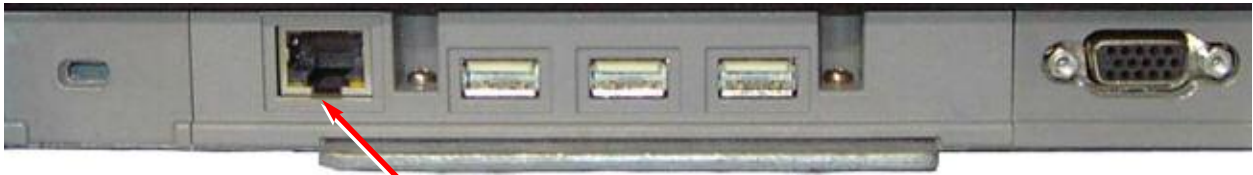
Docking station terminal strip (arrow pointing to RJ45 port)
