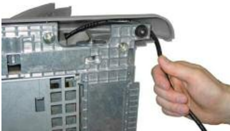
Power cable routing
