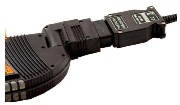
Connection of ICOM A with ICOM C
