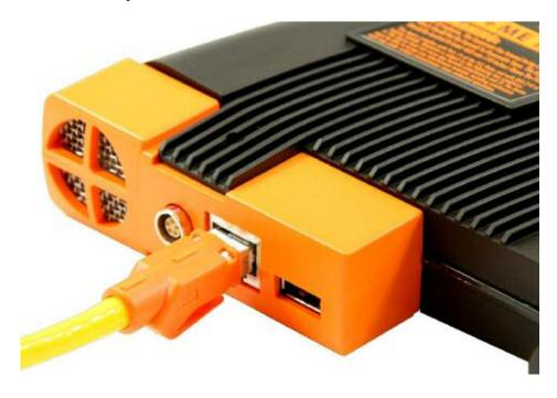
The IMIB can be connected by way of a LAN connector to the ICOM A.
