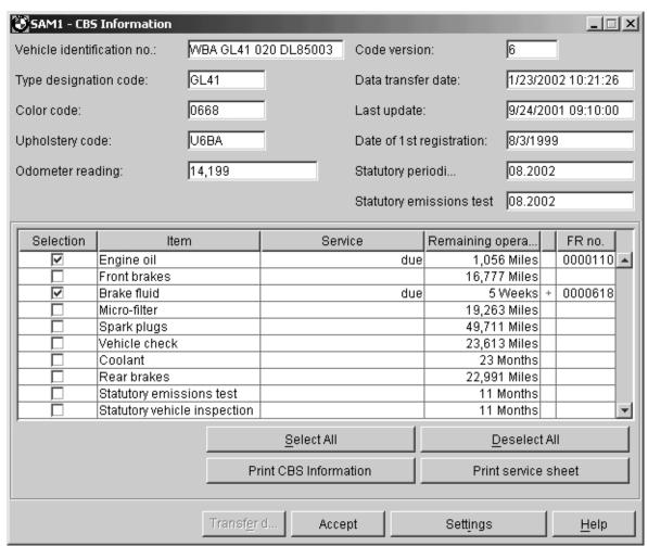
This on screen information provides the service advisor more specific information about the individual vehicle requirements when consulting with the customer. As shown above, the on screen information indicates that the engine oil and brake fluid is due to be changed. In addition, future service and maintenance requirements (based on mileage or time) can be planned.
