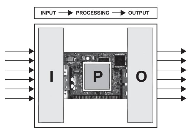
Any device controlled by a processor requires input to the alert the operating program of a condition. The program processes the input information and logically activates an output of a component.
