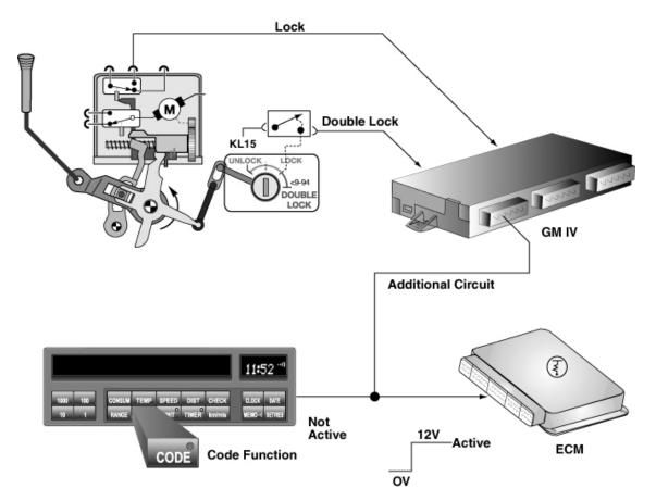
Note: The status pages of the ZKE and DME will show the condition of the Drive Away Protection signal as High/Active or Low/Not Active.
