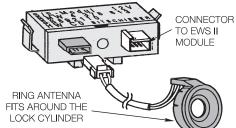
The transmitter/receiver module converts the analog data received through the AM signal to digital data and transfers it to the EWS II control module over a single wire bi-directional data interface.
