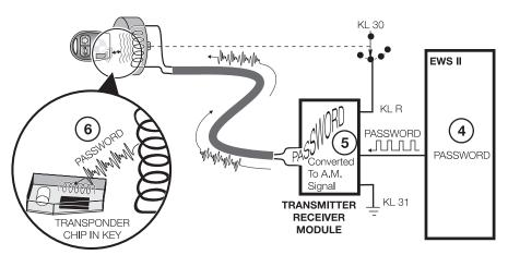
• If the transponder accepts the password as correct the transponder releases the changing code (7) to the transmitter/receiver module which converts this AM signal to digital (8) and sends it to the EWS II module (9).
