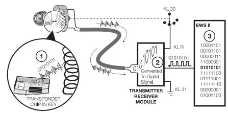
• Upon accepting the key as valid and enabled the EWS II control module sends a digital password (4) to the transmitter/receiver module, which converts the data to an AM signal (5) and sends it to the transponder via the ring antenna (6).
