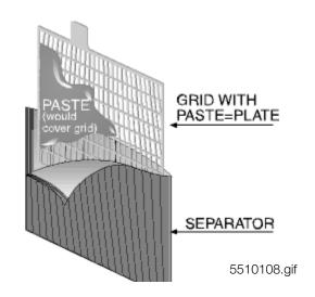
A forming charge is applied to the positive plates converting the Lead Oxide to Lead Dioxide, a highly porous material which allows the electrolyte to freely penetrate the plate. A forming charge is also applied to the negative plates converting the Lead Oxide to Sponge Lead. The Sponge Lead allows the electrolyte to penetrate freely allowing the material beneath the plate surface to take part in the chemical reaction.
