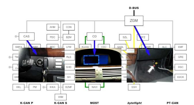
The CAS is the Gateway between the K-CAN System and K-CAN Periphery Bus.
