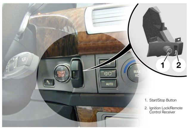
The ignition lock/start button (ZAS) is located in the instrument panel between the instrument cluster and the control display at the level of the trim strips.
