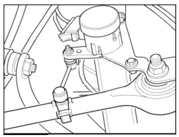
Note: E39 sport wagon vehicles with EHC have a dual output sensor at the right rear location. This sensor shares the same housing as the EHC systems right rear level sensor.
