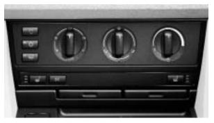
The E39 IHKR is a single zone system that regulates the temperature of the cabin based on the occupants desired temperature, selected by a temperature setting dial. Blower control, air distribution settings and stratification flap are manual.
