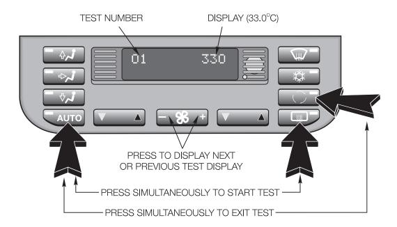
The sensor display mode is activated by pressing the "AUTO" and rear window defroster buttons simultaneously.
