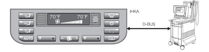
The IHKA control panel/module is coded with the central coding key (ZCS) using the DIS or MoDiC. The ZCS coding procedures is the same as on previous systems.
