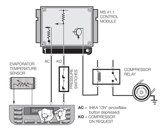
When A/C is requested (by pressing the "snowflake"), the IHKA control panel/module sends a request signal to the engine control module.
