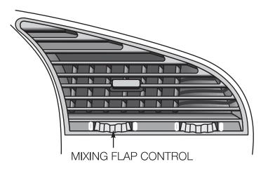
Any time that the face vents are open, rotating the thumbwheel will operate the mixing flap which is located above the space between the evaporator and the heater cores. Opening the mixing flap allows more cooled air to enter the face vent ductwork. Closing the flap increases the proportion of heated air which enters the face vent ductwork.
