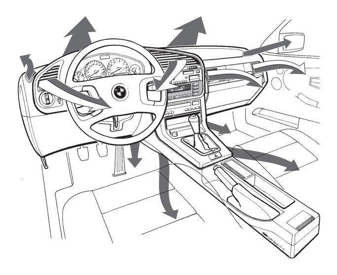
All outlet flaps are operated by M-bus stepper motors, controlled by the control panel/module:
