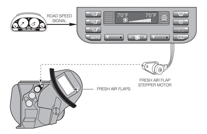
The fresh air flaps stepper motor operates only when the ignition switch is in "Run." At engine shut-down, the fresh air flaps stay in their "last-used" position. When the ignition switch is again turned to "Run," the control module/panel operates the stepper motor to move the flaps, if necessary.
