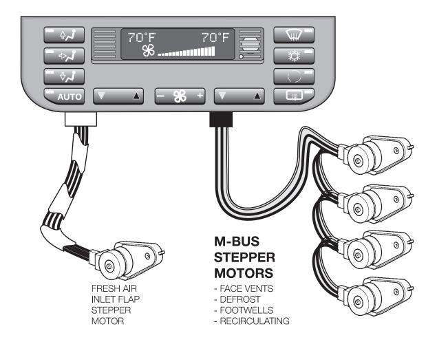
Like IHKA E38, IHKA E36 uses an M-Bus to control all stepper motors except the fresh air flaps stepper motor. IHKA E36, however, uses only five stepper motors:
