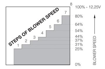
The control panel/module processes the blower speed rocker switch input and sends a signal to the final stage unit. The final stage unit then regulates blower motor voltage to control blower speed.
