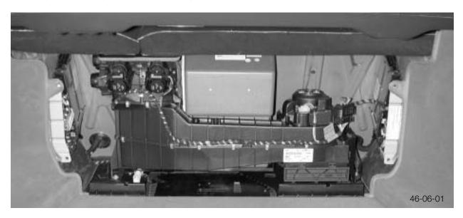
The control and integration of the rear compartment air conditioning system in the IHKA refrigerant circuit is designed so that independent operation is possible for either the front or rear unit.
