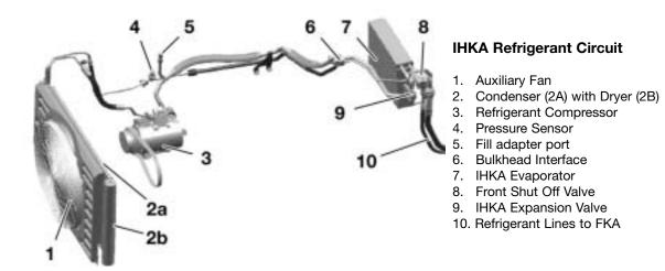
The rear compartment air conditioning system (FKA) is connected to the refrigerant circuit of the IHKA. The two circuits are isolated by means of two shut-off valves that are fitted only in connection with the rear compartment air conditioning system. The shut-off valves are fitted in the pressure line ahead of the respective expansion valves of IHKA and FKA.
