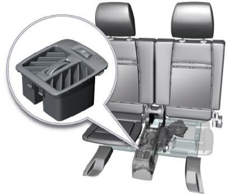
E70 HB3SR Vent and control location
