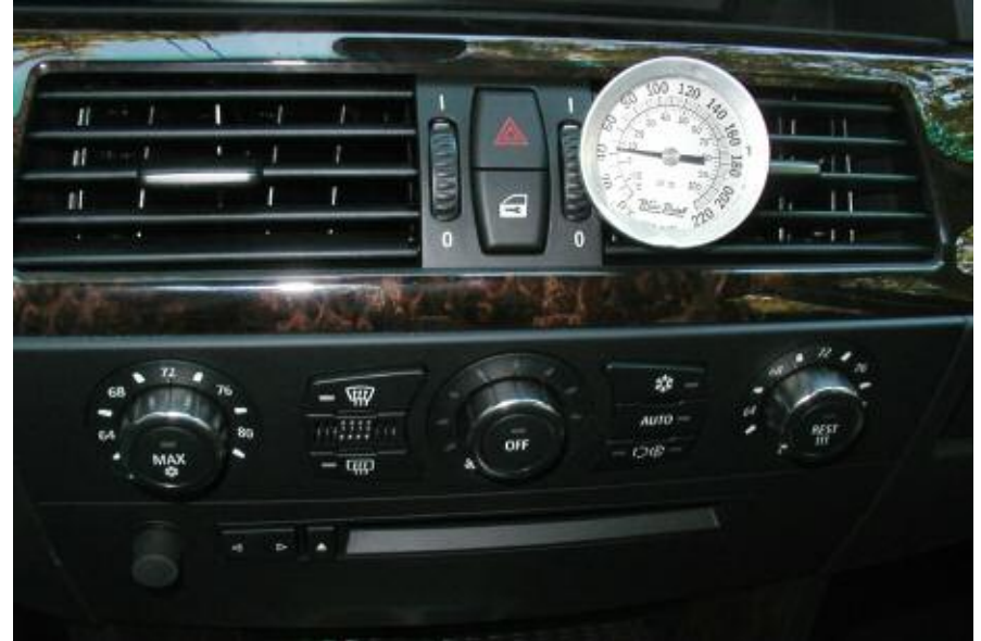
E60 vent outlet temperature reading
