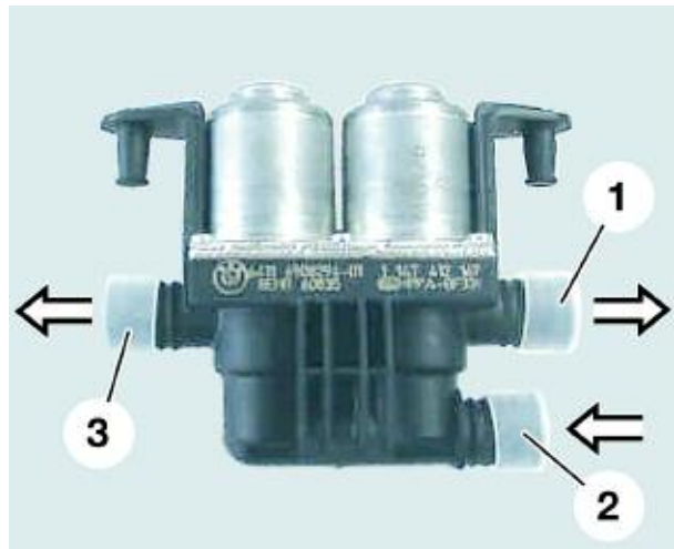
E65 Water Valve
