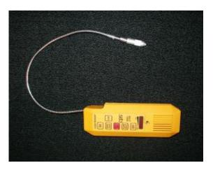
The tip of the detector can be inserted in and around the suspected refrigerant leaks like between condenser fins or the outlet vents on the dash or in the water drain hose of the evaporator box to check for a leaking evaporator. A downside to using this method would be that in some shops the service area may be contaminated with different gasses that make the tool a somewhat difficult to operate.
