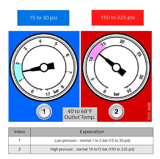
Outlet temperatures may vary from 40 to 68°F at any given time depending on ambient temperature and humidity. Readings of about 20° less than ambient temperatures are considered acceptable. Several fault symptoms involving high pressure and low pressure are described in the following examples, together with possible corrective measures.
