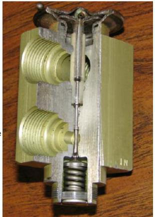
When the pressure at the evaporator outlet is high, this increases the pressure needed by the capillary tube to open the valve. Less refrigerant is provided to the evaporator (to prevent the evaporator from being flooded).
