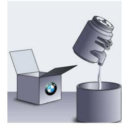
Depending on the version, the new compressor is filled with 120 to 200g of refrigerant oil at the factory.
