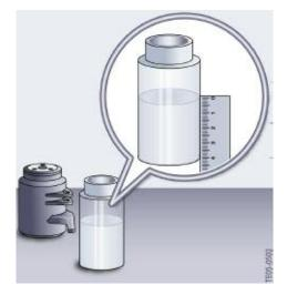
Measure the collected quantity of refrigerant oil from the old compressor.
