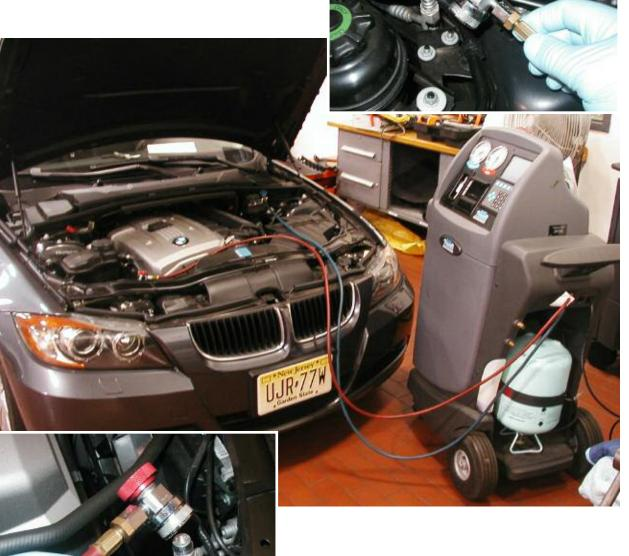
The High side hose is RED in color and also incorporates a quick disconnect type fitting along with a shut off valve so as to minimize refrigerant leakage.
