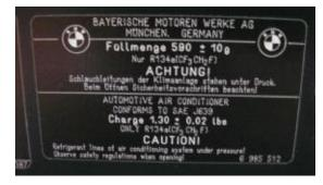
To determine the exact amount of refrigerant needed for the vehicle's air conditioning system, locate the label under the hood. The label specifies the type and quantity of refrigerant the system requires. This vehicle label calls for 1.30 + -0.02 lbs of R134a.
