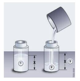
Using only new refrigerant oil, fill the same quantity as extracted from the old compressor + 10g safety amount into a clean measuring beaker and refill the new compressor. The remainder of the new refrigerant oil can be filled into the reservoir of the service station. Otherwise, the surplus refrigerant oil must be disposed of correctly.
