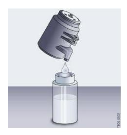
Empty the refrigerant oil remaining in the old compressor via the filler plug into a measuring beaker.
