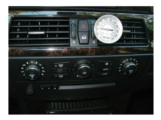
Typical Use: A/C Performance Quick Check Test conditions = 90°F & 50% Humidity
