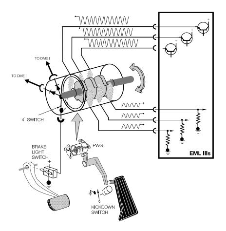
The amplitude is decreased as the pedal is pressed down.
