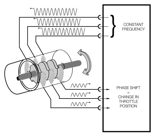
The changing amplitude value is a measure of accelerator pedal movement. The EML control module is programmed to recognize pedal movement from 0° (idle) to 99° (WOT) based on the changing voltage signal.
