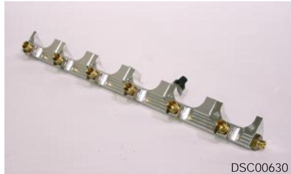
**Pressure Limiting Valves:** Each fuel rail contains an integral pressure limiting valve (1 below). This valve opens from a pressure of 125 bar to prevent damage to the injection system. The outlet of this valve is connected by a line to the high pressure pump fuel feed line. The valve can open briefly:
