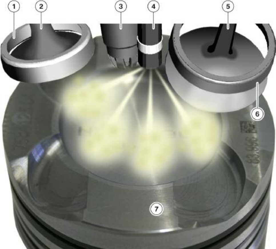
N55, combustion chamber with components
