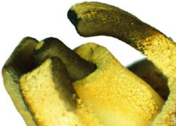
The spark plug above shows erosion of the electrode on one side and damage on the insulator nose. This could also be an indication of fuel spray "diversion".
