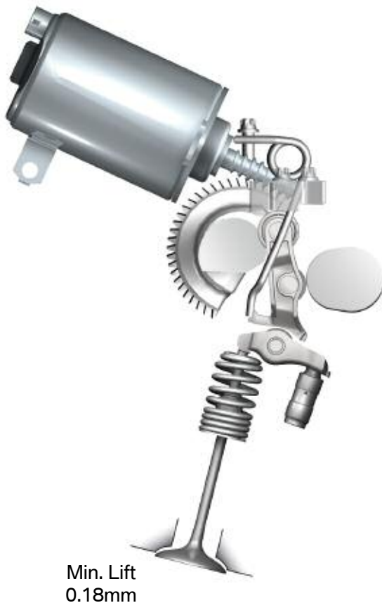
Valvetronic II at minimum valve lift
