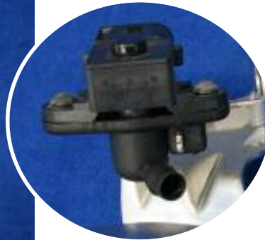
Secondary Air Valve and Pressure Sensor
