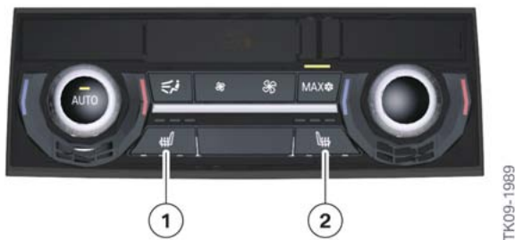
F10 Control panel for the rear IHKA
