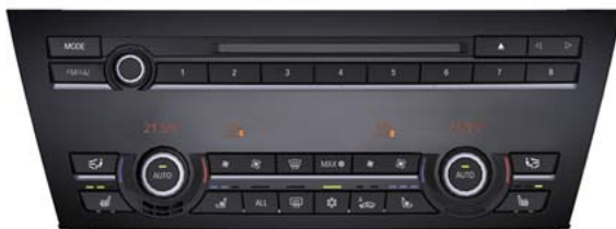
F10 Control panel of the 2-zone IHKA
