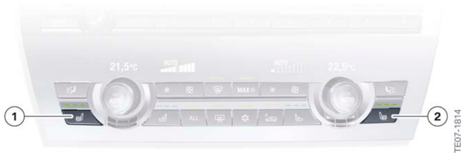
F10 Control panel for integrated automatic heating / air conditioning system
