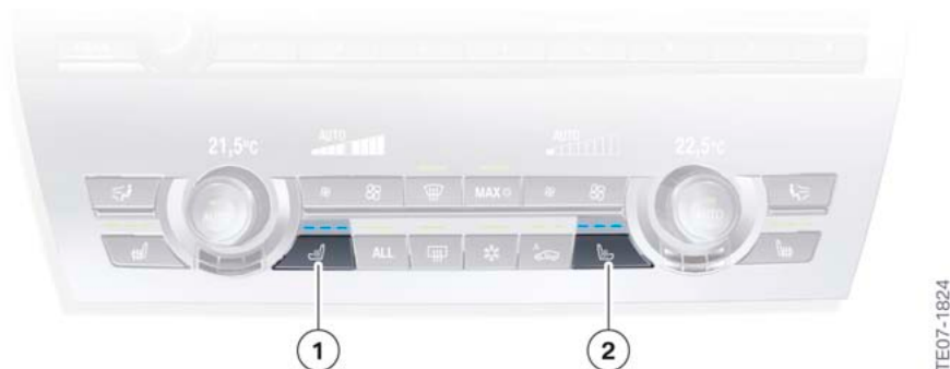
F10 Control panel for integrated automatic heating / air conditioning system
