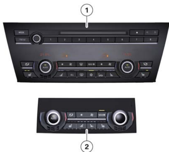
F10 Control panels for the 4-zone IHKA
